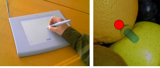
Figure 4. Pen angle is directly associated with the surface normal to allow intuitive normal painting. The cursor in the right image shows the angle of surface normal input.
