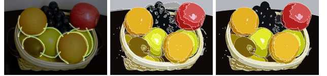
Figure 3. Important boundaries can be explicitly specified with a user input stroke. (From left to right) Left: User-defined rough strokes, Middle: segmentation result without strokes, and Right: segmentation result with strokes. Important boundaries are well preserved in the right image.
