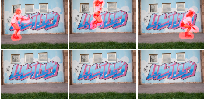
Fig. 6. It took 1 minute in total to remove the rollerblader from the 35-frame video with a resolution of 854 \times 480 pixels. The top row shows the user-drawn masks and the bottom row shows the frames of the completed video.
